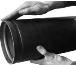
1.Pipe preparation Check pipe end for proper groove dimensions and to assure that pipe end is free of indentations and projections that would prevent proper sealing.
