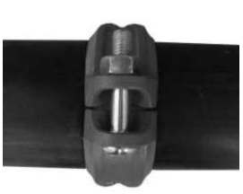
7 a.Assembly completed- Rigid Coupling For Rigid Coupling, keep the gaps at bolt pads evenly spaced. Gaskets can't be seen visually.
