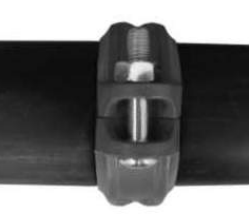
7 b. Assembly completed- Flexible Coupling For Flexible Coupling, two housings should be iron to iron connected. Gaskets can't be seen visually.
